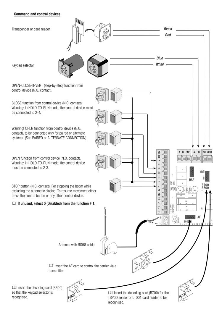
WARNING! To ensure correct operation, before inserting any plug-in card (e.g. AF, R800), LINE VOLTAGE MUST BE DISCONNECTED. If installed, disconnect the batteries.
