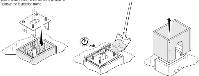
Fill the hole with earth around the concrete block.
