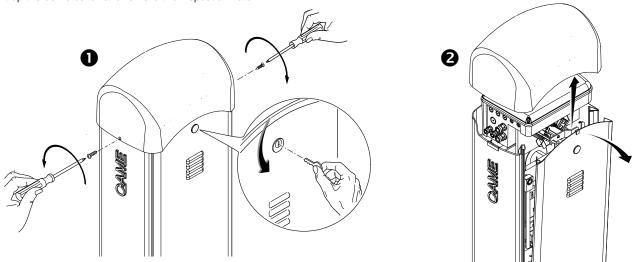
△ Caution! The barrier is set up for installing on the left. If it is installed on the right, invert the boom opening direction, following the procedure below:
