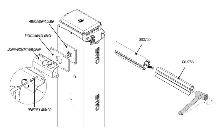
Fit the boom into the attachment cover and fasten it using the screws.
