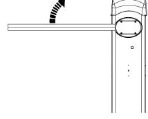
Before calibrating the travel, identify the type of boom, check that the boom is balanced and check that the manoeuvring area is clear of any obstacles.
