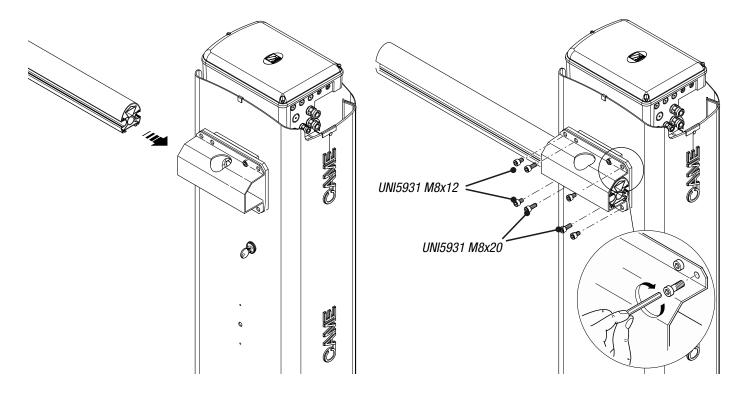
Cut the groove covers to the required length and insert them in the boom conduits on both sides  $\odot$ 2. Insert the shockproof rubber profile in the boom and cut off the excess  $\odot$ .
