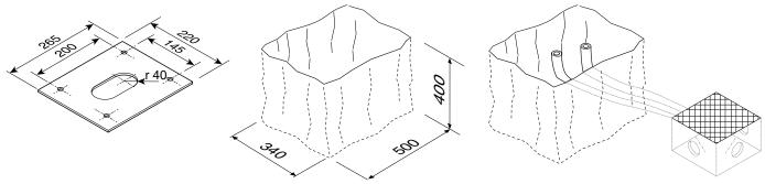
Prepare a foundation frame that is larger than the anchoring plate and sink it into the dug hole.
