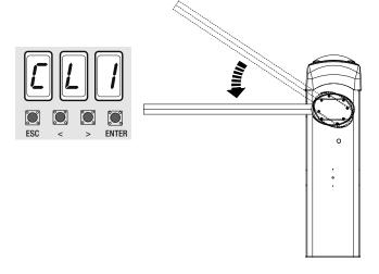
4. ...then the operator opens until it reaches the limit-switch point.
