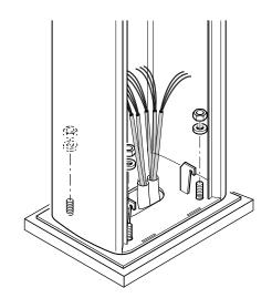
Attach the intermediate plate and boom-attachment cover to the attachment plate with a screw. Leave the screw loose to make it easier to insert the boom.
